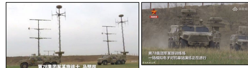
(U) Hybrid RF jamming and RDF platforms, mast-mounted on CTL-181 tactical wheeled vehicles. These are example of systems deployed to forward areas.
